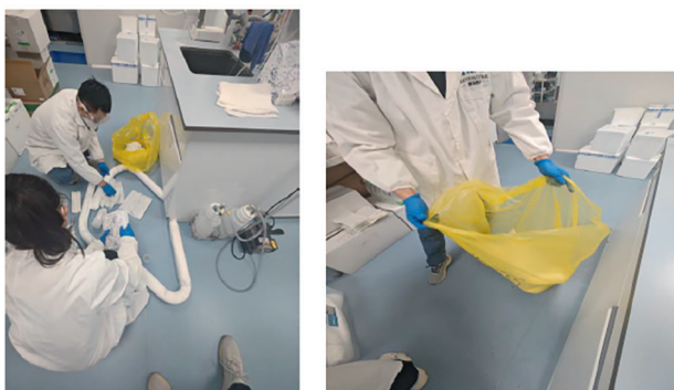
Emergency response team handled spilled chemicals on site (left) and collected the treated waste into hazardous waste storage bags (right)
